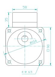
Motor Round Shaft with Terminal Box
