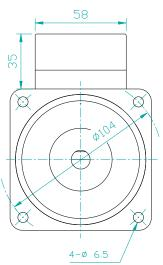
Motor, Gearbox with Lead Wires
